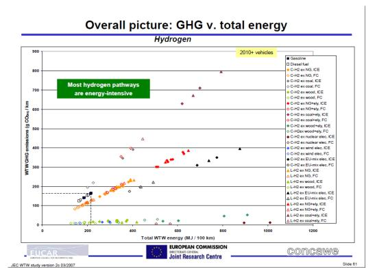
**Fig. 9:** CO<sub>2</sub> emissions versus energy consumption for hydrogen powered vehicles over the whole fuel chain for different hydrogen production pathways (JEC Well-To-Wheels study, Version 2c, March 2007)
