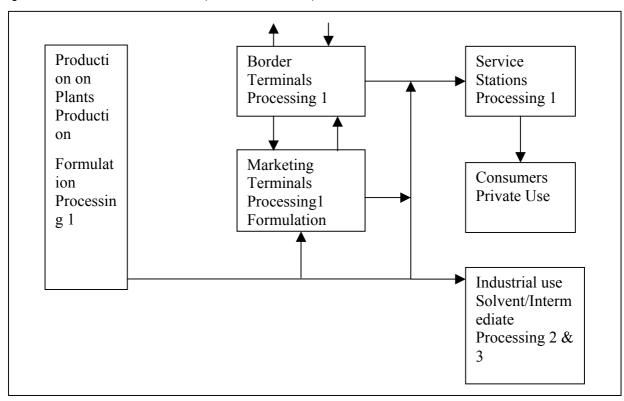
Figure 1 Basic MTBE material flowchart (emission flows omitted)
