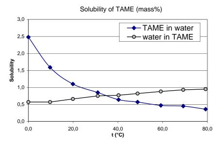
If water solubility is extrapolated to 12°C, the relevant temperature for the regional model, approximately 15 g/l is the approximate result from **Figure 1.2** above.
