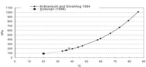
Figure 1.1 Vapour pressure of TAME at different temperatures. Data from Huttunen (1996) and (Krähenbül and Gmehling 1994)
